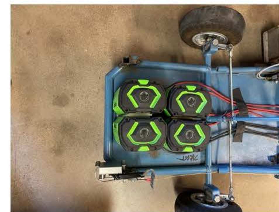
Figure 5. Last Years Battery Mount
