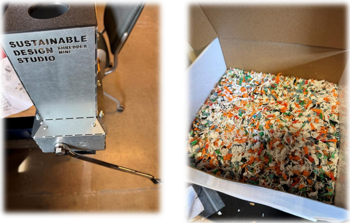
Figure 6: (Left) Shredder turned by using 19mm wrench, (Right) Box of shredded filament
