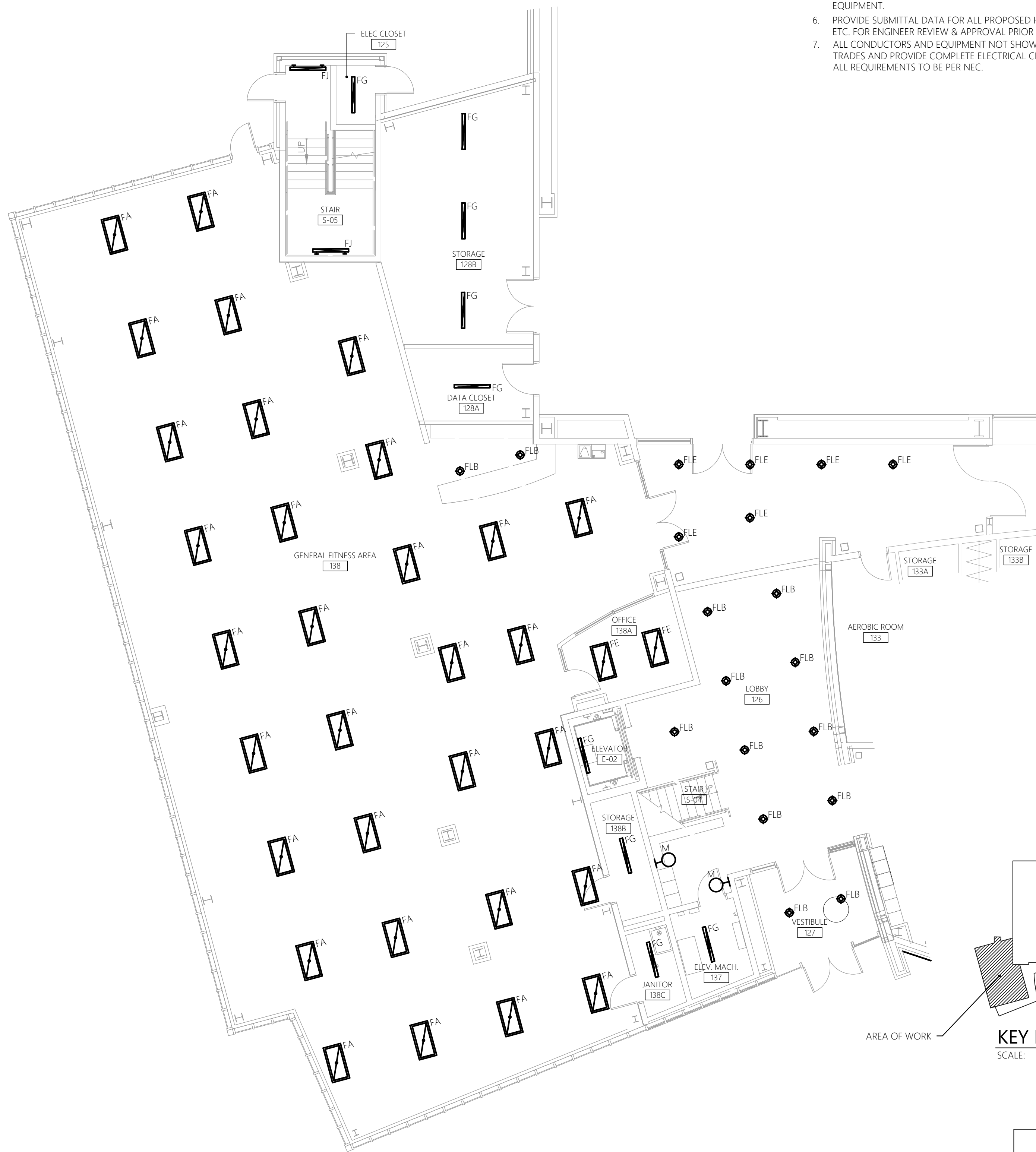
1 ELECTRICAL LIGHTING PLAN SCALE: 1/8" = 1'-0" 1ST FLOOR
